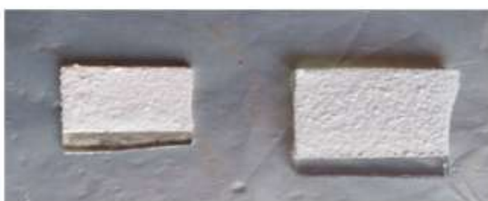
Figure: 1. Coating of \text{TiO}_2 nano particles using Doctor Blade Method.
