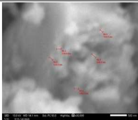
a) SEM micrographs of TiO 2 Nanoparticles synthesized via Sol-Gel method
